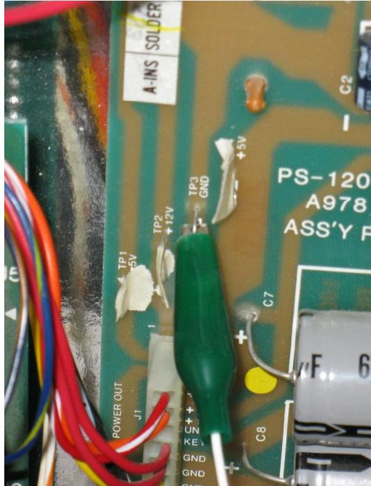
**\*\*\*LaserCon has a redundant ground loop through the player cable and audio jacks. Connecting the alligator clip to any test point other than GND will blow fuses.\***
