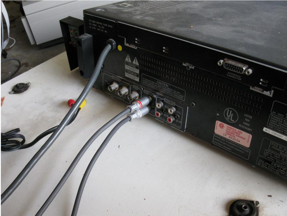
Attach "Audio Out (L and R)" to the GSI board.
