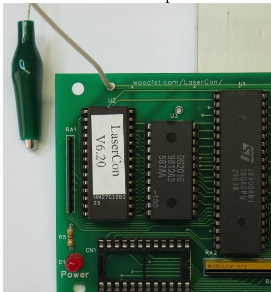
Find the +5Volt test loop on the power supply board.
