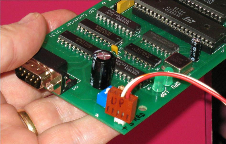
\*\*\* +5Volts is supplied to the LaserCon board through this connector.
