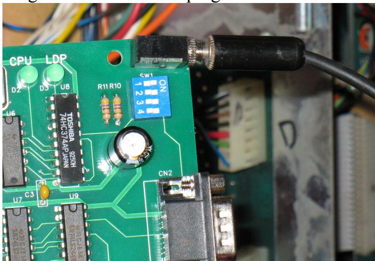
In Direct Wire mode, your LaserCon board needs to connect to +5Volts.
